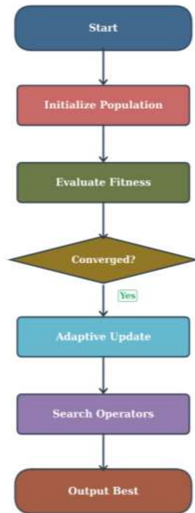
Fig. 1. Workflow of the ASD-HHS algorithm. The adaptive update loop adjusts search parameters based on population entropy, while the convergence check terminates the search when improvement falls below a threshold.
